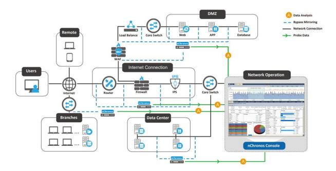
To capture traffic effectively, the traffic sources are must from appropriate network devices. Managed switches are the perfect choice because you can use their port mirroring/SPAN function to copy the packets to a monitor port. This function is called as *Port Mirroring* (Cisco calls it *SPAN*).
