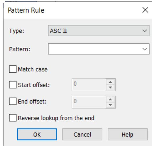
The unit for offset is byte.
