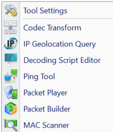
In tools menu, users can use built-in network tools, codec transform, IP geolocation query, decoding script editor, ping tool, packet player, packet builder and MAC scanner are included. Go to [Network Tools](#) for more information.
