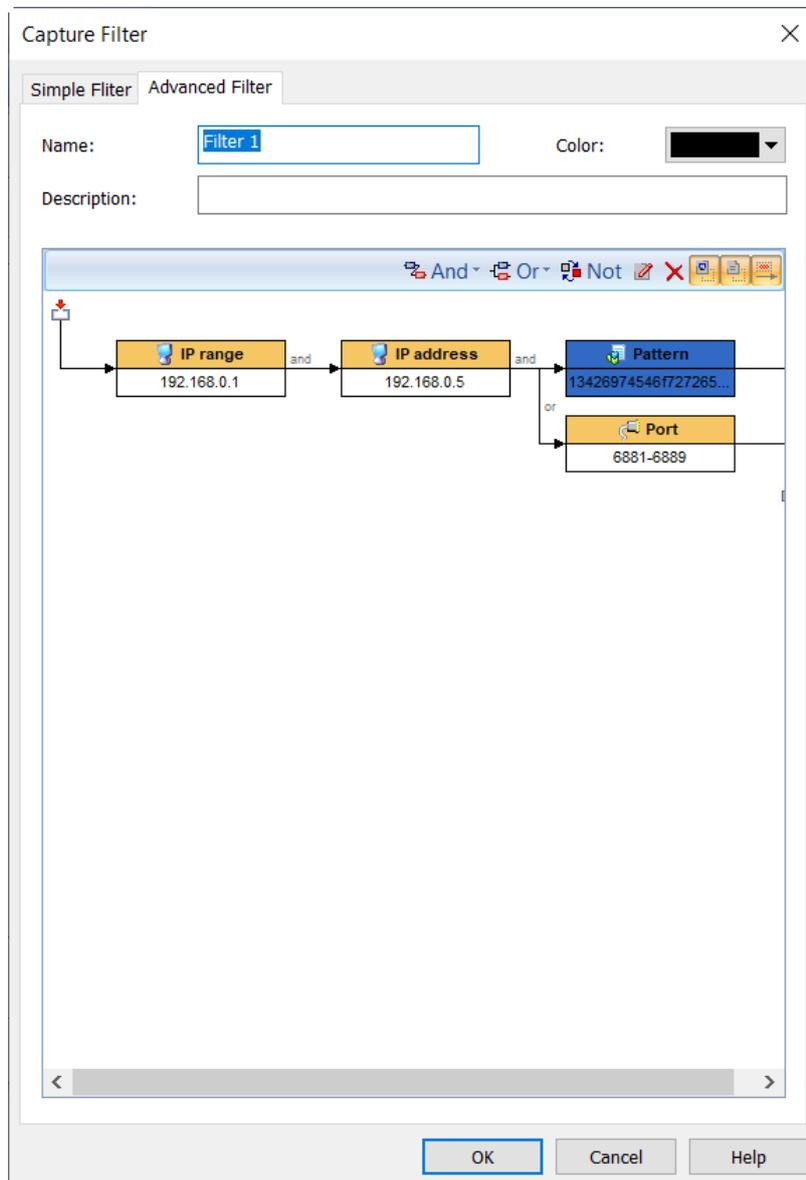
The filter rules are arranged in a filter relation map. The map shows the logical relations among the rules from adapter to an analysis project. You can double-click the rule to edit it.
