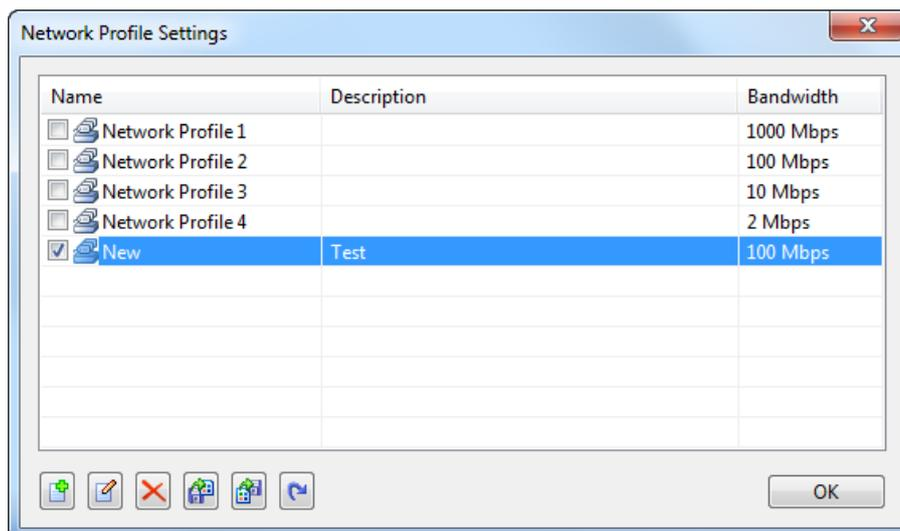
The **Network Profile Settings** dialog box includes all available network profiles. You can use the buttons on the bottom of the dialog box to add, edit and delete a network profile, or import/export a network profile file.
