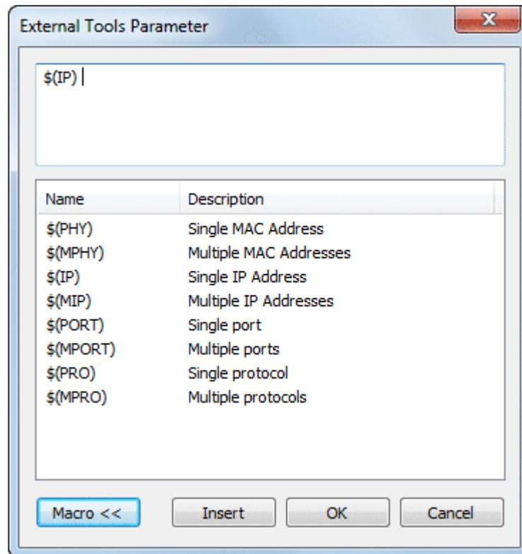
Colasoft Capsa lists the parameters IP Address, Physical Address, Port and Protocol in the window. You can add a parameter by selecting its name and clicking the Insert button. If the parameters are not listed, you can enter the parameters into the upper window manually, like as -d, -h, -j and -w in Tracert command. Every parameter should be separated with a blank space.
