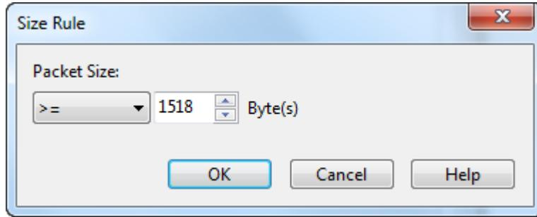
You can choose < (less than), <= (less than or equal to), > (greater than), >= (greater than or equal to), = (equal to), != (not equal to), Between (size range) to define the size rule.
