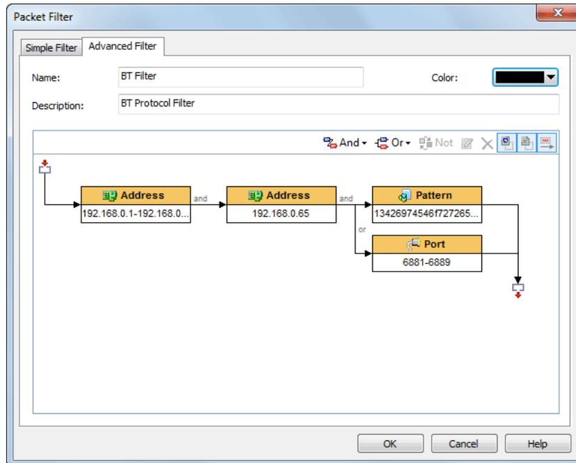
The filter rules are arranged in a filter relation map. The map shows the logical relations among the rules from adapter to an analysis project. You can double-click the rule to edit it.
