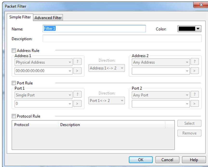
The **Simple Filter** tab allows you to create simple filters by address, port and protocol. When multiple parameters are set, they are connected by logical AND statements. That is, packets must match all of the conditions to match the filter.
